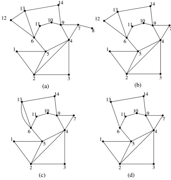
Fig. 2: A simple diagram illustrating a sequence of series-parallel reductions for the IEEE 14-bus system.
