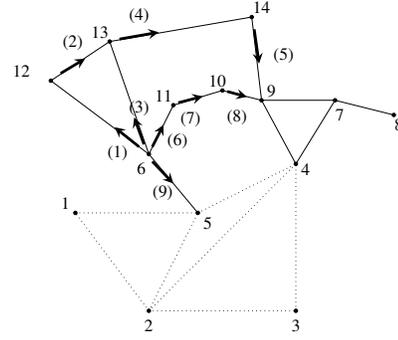
Fig. 4: A simple diagram of the IEEE 14-bus system. Buses are marked in plain numbers, while the flow variables are marked in parenthesized numbers in the order in which they are calculated in Algorithm 1. Nodal real power injections are not shown in order to simplify the diagram.
