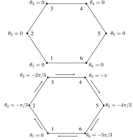
Fig. 1: Cycle example showing multiple solutions. The two graphs show two different solutions that satisfy the power flow equations. In the top solution, there is no flow going around the cycle. In the bottom solution, there is a clockwise flow going around the cycle.
